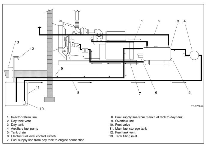
Figure 6-1 Diesel Fuel System
